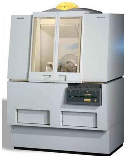
**Figure 2.12:** The XRD instrument used for measuring the spectra.
