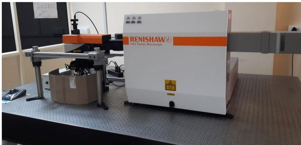
**Figure 2.11:** The Laser Raman instrument used for measuring the spectra.
