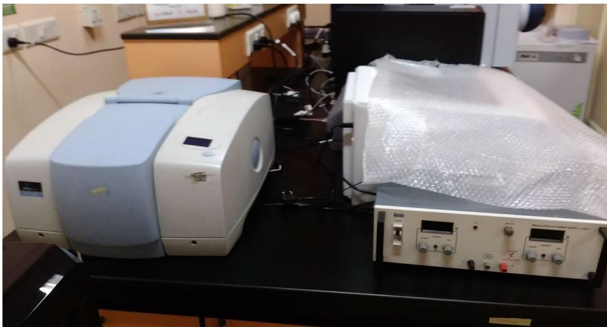
**Figure 2.10:** The FTIR instrument used for measuring the absorbance spectra.
